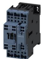
power contactor, AC-3e/AC-3, 25 A, 11 kW / 400 V, 3-pole, 110 V AC, 50 Hz / 120 V, 60 Hz, auxiliary contacts: 1 NO + 1 NC, spring-loaded terminal, size: S0
