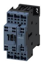
power contactor, AC-3e/AC-3, 25 A, 11 kW / 400 V, 3-pole, 110 V AC, 50 Hz / 120 V, 60 Hz, auxiliary contacts: 1 NO + 1 NC, spring-loaded terminal, size: S0, upright mounting position
