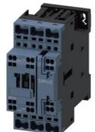
power contactor, AC-3e/AC-3, 25 A, 11 kW / 400 V, 3-pole, 24 V AC, 50/60 Hz, auxiliary contacts: 1 NO + 1 NC, spring-loaded terminal, size: S0
