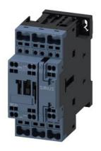
power contactor, AC-3e/AC-3, 25 A, 11 kW / 400 V, 3-pole, 24 V AC, 50 Hz, auxiliary contacts: 1 NO + 1 NC, spring-loaded terminal, size: S0, upright mounting position
