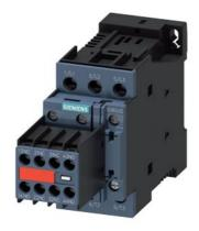
power contactor, AC-3e/AC-3, 25 A, 11 kW / 400 V, 3-pole, 24 V DC, with plugged-in varistor, auxiliary contacts: 2 NO + 2 NC, screw terminal, size: S0, captive auxiliary switch
