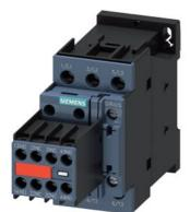
power contactor, AC-3e/AC-3, 25 A, 11 kW / 400 V, 3-pole, 230 V AC, 50/60 Hz, with plugged-in varistor, auxiliary contacts: 2 NO + 2 NC, screw terminal, size: S0, captive auxiliary switch
