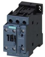
power contactor, AC-3e/AC-3, 25 A, 11 kW / 400 V, 3-pole, 125 V DC, auxiliary contacts: 1 NO + 1 NC, screw terminal, size: S0
