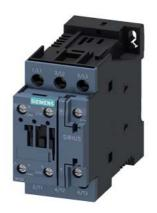
power contactor, AC-3e/AC-3, 25 A, 11 kW / 400 V, 3-pole, 24 V DC, auxiliary contacts: 1 NO + 1 NC, screw terminal, size: S0, communication-capable
