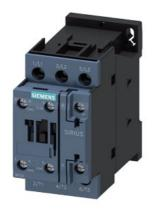
power contactor, AC-3e/AC-3, 25 A, 11 kW / 400 V, 3-pole, 220 V AC, 50 Hz / 240 V, 60 Hz, auxiliary contacts: 1 NO + 1 NC, screw terminal, size: S0
