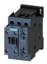
power contactor, AC-3e/AC-3, 25 A, 11 kW / 400 V, 3-pole, 220 V AC, 50/60 Hz, auxiliary contacts: 1 NO + 1 NC, screw terminal, size: S0  $\,$
