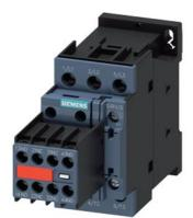
power contactor, AC-3e/AC-3, 25 A, 11 kW / 400 V, 3-pole, 230 V AC, 50/60 Hz, auxiliary contacts: 2 NO + 2 NC, screw terminal, size: S0, captive auxiliary switch, no surge suppressor retrofittable
