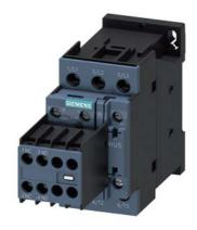
power contactor, AC-3e/AC-3, 25 A, 11 kW / 400 V, 3-pole, 110 V AC, 50/60 Hz, auxiliary contacts: 2 NO + 2 NC, screw terminal, size: S0, removable auxiliary switch
