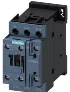
power contactor, AC-3e/AC-3, 25 A, 11 kW / 400 V, 3-pole, 110 V AC, 50 Hz, auxiliary contacts: 1 NO + 1 NC, screw terminal, size: S0
