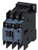
traction contactor, AC-3e/AC-3, 17 A, 7.5 kW / 400 V, 3-pole, 24 V DC, 0.7-1.25\* Us, electronic drive, with integrated varistor, auxiliary contacts: 1 NO + 1 NC, ring cable lug connection, size: S0
