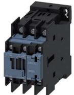
power contactor, AC-3e/AC-3, 17 A, 7.5 kW / 400 V, 3-pole, 24 V DC, auxiliary contacts: 1 NO + 1 NC, ring cable lug connection, size: S0
