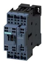
traction contactor, AC-3e/AC-3, 17 A, 7.5 kW / 400 V, 3-pole, 110 V DC, 0.7-1.25\* Us, electronic drive, with integrated varistor, auxiliary contacts: 1 NO + 1 NC, spring-loaded terminal, size: S0
