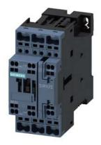
power contactor, AC-3e/AC-3, 17 A, 7.5 kW / 400 V, 3-pole, 24 V DC, 0.7-1.25\* Us, with plugged-in varistor, auxiliary contacts: 1 NO + 1 NC, spring-loaded terminal, frame size: S0, suitable for PLC outputs, not expandable with auxiliary switch expandable
