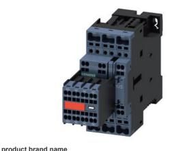
power contactor, AC-3e/AC-3, 17 A, 7.5 kW / 400 V, 3-pole, 24 V DC, with plugged-in diode combination, auxiliary contacts: 2 NO + 2 NC, spring-loaded terminal, size: S0, captive auxiliary switch
