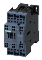
power contactor, AC-3e/AC-3, 17 A, 7.5 kW / 400 V, 3-pole, 230 V DC, auxiliary contacts: 1 NO + 1 NC, spring-loaded terminal, size: S0  $\,$
