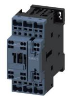
power contactor, AC-3e/AC-3, 17 A, 7.5 kW / 400 V, 3-pole, 230 V AC, 50 Hz, auxiliary contacts: 1 NO + 1 NC, spring-loaded terminal, size: S0, upright mounting position
