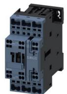
power contactor, AC-3e/AC-3, 17 A, 7.5 kW / 400 V, 3-pole, 110 V AC, 50 Hz / 120 V, 60 Hz, auxiliary contacts: 1 NO + 1 NC, spring-loaded terminal, size: S0
