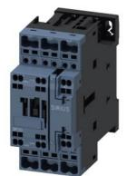
power contactor, AC-3e/AC-3, 17 A, 7.5 kW / 400 V, 3-pole, 110 V AC, 50 Hz / 120 V, 60 Hz, auxiliary contacts: 1 NO + 1 NC, spring-loaded terminal, size: S0, multi-unit packaging, pack = 18 units
