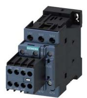
power contactor, AC-3e/AC-3, 17 A, 7.5 kW / 400 V, 3-pole, 24 V DC, with plugged-in diode combination, auxiliary contacts: 3 NO + 2 NC, screw terminal, size: S0, with 3RH2911-1HA21
