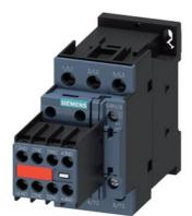
power contactor, AC-3e/AC-3, 17 A, 7.5 kW / 400 V, 3-pole, 110 V AC, 50 Hz / 120 V, 60 Hz, with plugged-in varistor, auxiliary contacts: 2 NO + 2 NC, screw terminal, size: S0, captive auxiliary switch
