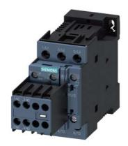
power contactor, AC-3e/AC-3, 17 A, 7.5 kW / 400 V, 3-pole, 24 V DC, auxiliary contacts: 2 NO + 2 NC, screw terminal, size: S0, removable auxiliary switch
