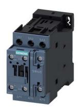
power contactor, AC-3e/AC-3, 17 A, 7.5 kW / 400 V, 3-pole, 24 V DC, auxiliary contacts: 1 NO + 1 NC, screw terminal, size: S0, communication-capable
