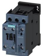
power contactor, AC-3e/AC-3, 17 A, 7.5 kW / 400 V, 3-pole, 600 V AC, 60 Hz, auxiliary contacts: 1 NO + 1 NC, screw terminal, size: S0
