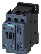
power contactor, AC-3e/AC-3, 17 A, 7.5 kW / 400 V, 3-pole, 200 V AC, 50 Hz / 200-220 V, 60 Hz, auxiliary contacts: 1 NO + 1 NC, screw terminal, size: S0
