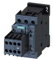
power contactor, AC-3e/AC-3, 17 A, 7.5 kW / 400 V, 3-pole, 230 V AC, 50/60 Hz, auxiliary contacts: 2 NO + 2 NC, screw terminal, size: S0, removable auxiliary switch
