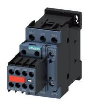
power contactor, AC-3e/AC-3, 17 A, 7.5 kW / 400 V, 3-pole, 230 V AC, 50/60 Hz, auxiliary contacts: 2 NO + 2 NC, screw terminal, size: S0, captive auxiliary switch, no surge suppressor retrofittable
