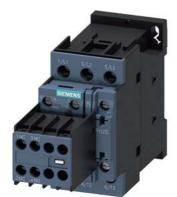
power contactor, AC-3e/AC-3, 17 A, 7.5 kW / 400 V, 3-pole, 110 V AC, 50/60 Hz, auxiliary contacts: 2 NO + 2 NC, screw terminal, size: S0, removable auxiliary switch
