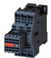
power contactor, AC-3e/AC-3, 12 A, 5.5 kW / 400 V, 3-pole, 24 V DC, with plugged-in varistor, auxiliary contacts: 2 NO + 2 NC, spring-loaded terminal, size: S0, captive auxiliary switch
