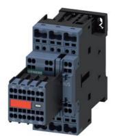
power contactor, AC-3e/AC-3, 12 A, 5.5 kW / 400 V, 3-pole, 230 V AC, 50/60 Hz, with plugged-in varistor, auxiliary contacts: 2 NO + 2 NC, spring-loaded terminal, size: S0, captive auxiliary switch
