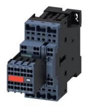
power contactor, AC-3e/AC-3, 12 A, 5.5 kW / 400 V, 3-pole, 24 V DC, auxiliary contacts: 2 NO + 2 NC, spring-loaded terminal, size: S0, captive auxiliary switch, no surge suppressor retrofittable
