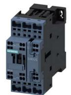
power contactor, AC-3e/AC-3, 12 A, 5.5 kW / 400 V, 3-pole, 24 V DC, auxiliary contacts: 1 NO + 1 NC, spring-loaded terminal, size: S0
