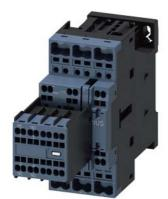
power contactor, AC-3e/AC-3, 12 A, 5.5 kW / 400 V, 3-pole, 220 V AC, 50/60 Hz, auxiliary contacts: 2 NO + 2 NC, spring-loaded terminal, size: S0, removable auxiliary switch
