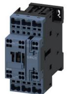
power contactor, AC-3e/AC-3, 12 A, 5.5 kW / 400 V, 3-pole, 110 V AC, 50/60 Hz, auxiliary contacts: 1 NO + 1 NC, spring-loaded terminal, size: S0
