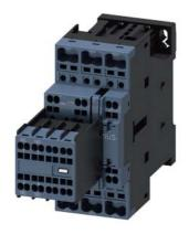
power contactor, AC-3e/AC-3, 12 A,  $5.5\,kW$  / 400 V, 3-pole, 24 V AC, 50/60 Hz, auxiliary contacts: 2 NO + 2 NC, spring-loaded terminal, size: S0, removable auxiliary switch
