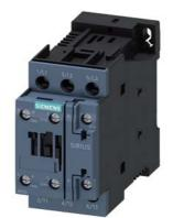
power contactor, AC-3e/AC-3, 12 A, 5.5 kW / 400 V, 3-pole, 24 V DC, 0.7-1.25\* Us, with plugged-in varistor, auxiliary contacts: 1 NO + 1 NC, screw terminal, size: S0, suitable for PLC outputs, not expandable with auxiliary switch , upright mounting position
