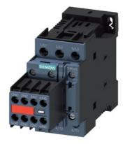
power contactor, AC-3e/AC-3, 12 A, 5.5 kW / 400 V, 3-pole, 24 V DC, with plugged-in diode combination, auxiliary contacts: 2 NO + 2 NC, screw terminal, size: S0, captive auxiliary switch
