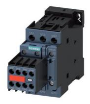
power contactor, AC-3e/AC-3, 12 A, 5.5 kW / 400 V, 3-pole, 24 V DC, with plugged-in varistor, auxiliary contacts: 2 NO + 2 NC, screw terminal, size: S0, captive auxiliary switch
