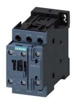
power contactor, AC-3e/AC-3, 12 A, 5.5 kW / 400 V, 3-pole, 24 V DC, with plugged-in varistor, auxiliary contacts: 1 NO + 1 NC, screw terminal, size: S0  $\,$
