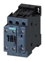
power contactor, AC-3e/AC-3, 12 A, 5.5 kW / 400 V, 3-pole, 24 V DC, auxiliary contacts: 1 NO + 1 NC, screw terminal, size: S0, upright mounting position
