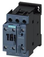
power contactor, AC-3e/AC-3, 12 A, 5.5 kW / 400 V, 3-pole, 110 V AC, 50 Hz / 120 V, 60 Hz, auxiliary contacts: 1 NO + 1 NC, screw terminal, size: S0
