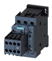
power contactor, AC-3e/AC-3, 12 A, 5.5 kW / 400 V, 3-pole, 42 V AC, 50 Hz, auxiliary contacts: 2 NO + 2 NC, screw terminal, size: S0, removable auxiliary switch
