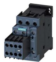
power contactor, AC-3e/AC-3, 12 A, 5.5 kW / 400 V, 3-pole, 24 V AC, 50 Hz, auxiliary contacts: 2 NO + 2 NC, screw terminal, size: S0, removable auxiliary switch
