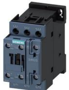
power contactor, AC-3e/AC-3, 12 A, 5.5 kW / 400 V, 3-pole, 24 V AC, 50 Hz, auxiliary contacts: 1 NO + 1 NC, screw terminal, size: S0
