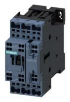
power contactor, AC-3e/AC-3, 9 A, 4 kW / 400 V, 3-pole, 24 V DC, with plugged-in diode combination, auxiliary contacts: 1 NO + 1 NC, spring-loaded terminal, size: S0
