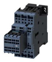
power contactor, AC-3e/AC-3, 9 A, 4 kW / 400 V, 3-pole, 24 V DC, auxiliary contacts: 2 NO + 2 NC, spring-loaded terminal, size: S0, removable auxiliary switch
