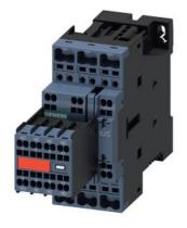
power contactor, AC-3e/AC-3, 9 A, 4 kW / 400 V, 3-pole, 24 V DC, auxiliary contacts: 2 NO + 2 NC, spring-loaded terminal, size: S0, captive auxiliary switch, no surge suppressor retrofittable
